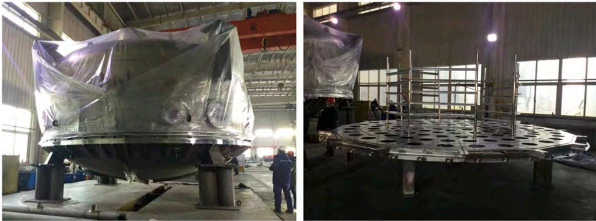
Figure 7.9: (Left) The aluminumizing chamber joining upper part and lower lid. (Right) Inside floor of the chamber. The filaments are set on the floor and covered by dedicated box.
