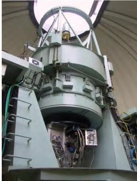
Figure 7.16: NICE at the Cassegrain focus of the 1.5m infrared telescope of National Astronomical Observatory of Japan.
