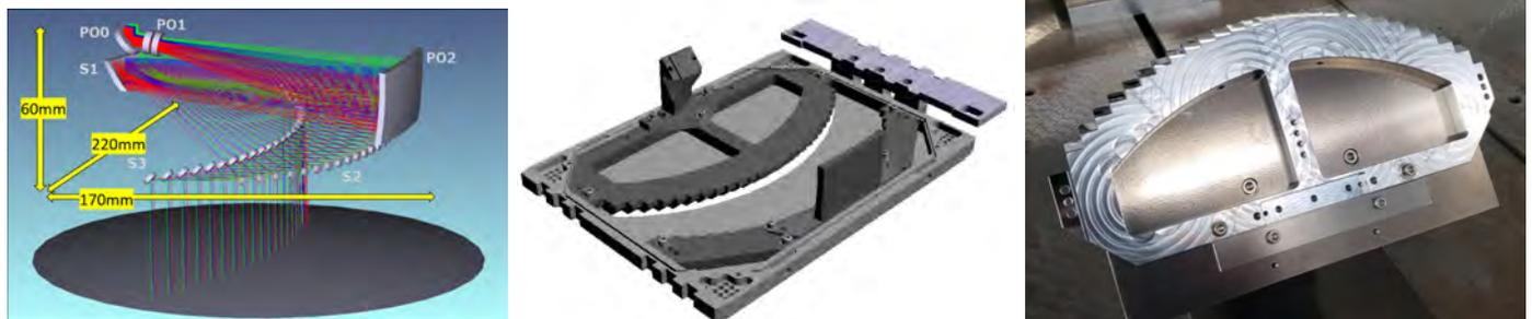
Figure 5.28: Left : Optical layout of SWIMS-IFU. The size of the optics is strongly limited by the dimension of the storage of SWIMS. Middle : Mechanical layout of SWIMS-IFU. Right : Fabricated slit-mirror array (S3).
