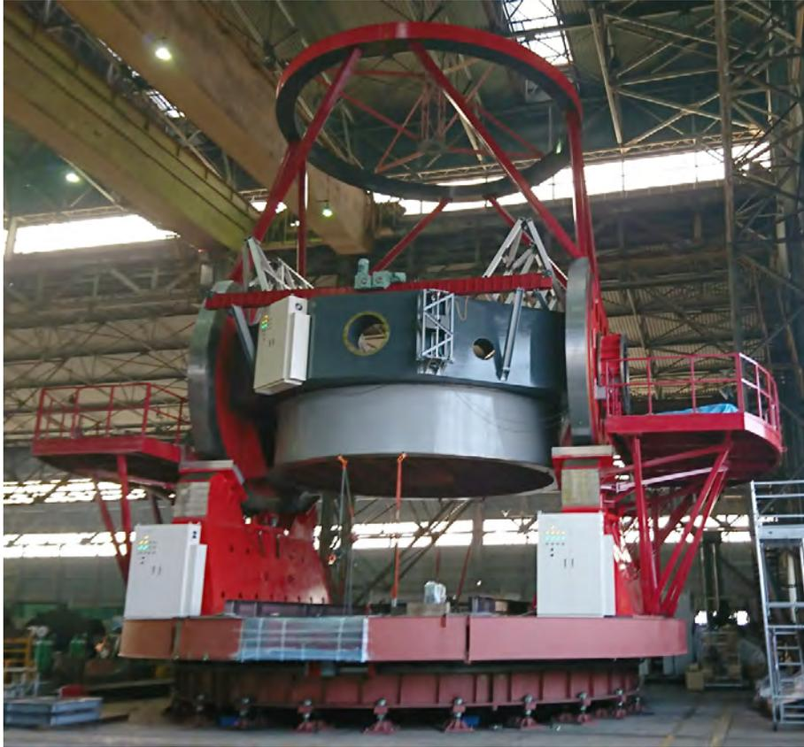
Figure 7.4: The telescope mount preassembled in Japan.
