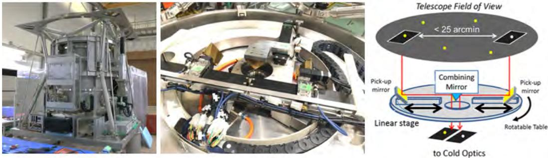
Figure 7.14: (Left) External view of MIMIZUKU. (Middle) The field stacker unit installed on the top of MIMIZUKU dewar. (Right) Principle of the field stacker.
