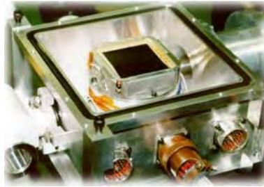
Figure 6.2: The 2K-CCD camera with the dewar opened.
