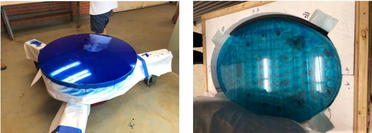
Figure 7.3: The aluminized secondary (left panel) and tertiary (right panel) mirrors. The blue film is for protection during the transportation.
