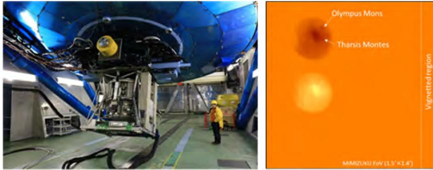
Figure 7.15: (Left) MIMIZUKU installed on the Subaru telescope. (Right) 10- $\mu\text{m}$  image of Mars.
