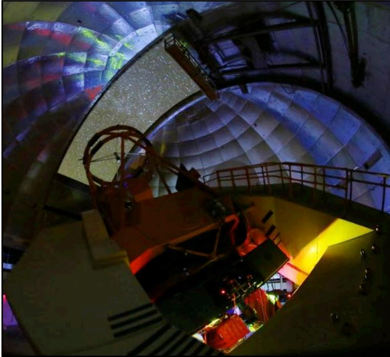
Telescope at night. At thermal infrared wavelengths ( $\lambda > 2.5 \mu\text{m}$ ), everything you see in this picture is bright, including the sky.
