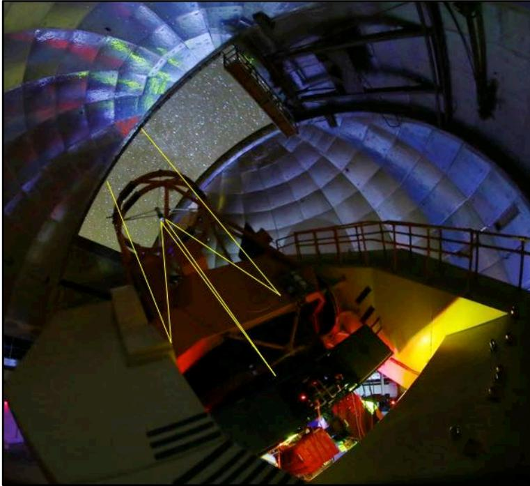
The light path is shown. Since the IRTF was designed to be a low infrared background telescope, the secondary mirror is very small. The focal ratio at the cassegrain focus is  $f/35$ . This minimizes the central obscuration and keeps the overall emissivity of the telescope low.
