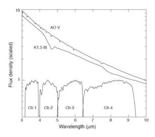
The Infrared Array Camera (IRAC) is a 4-channel camera operating at 3.6, 4.5, 5.8, and 8.0  $\mu$ m (Fazio et al. 2004). When the cryogens ran out in 2009, the observatory was operated using only the near-IR instrument at 3.6 and 4.5  $\mu$ m.
