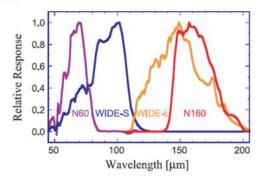
The figures show the filters for the Infrared Camera (IRC) on AKARI (Onaka et al. 2007) and the filters for the Far-Infrared Surveyor (FIS; Kawada et al. 2007).
