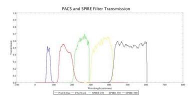
PACS AND SPIRE filters for imaging. The calibration of PACS is based on stars (Balog et al. 2014) while that for SPIRE is based on Neptune (Bendo et al. 2013). Figure is from Marston & Puga (2012).
