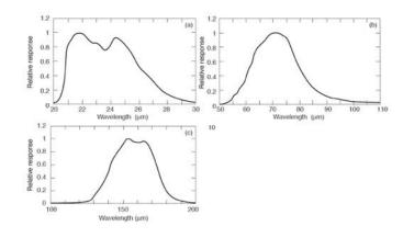
Figure shows the filters used for MIPS. Three types of detectors were used: a Si:As impurity band conduction array at 24  $\mu$ m (Rieke et al. 2008), a Ge:Ga photoconductor array at 70  $\mu$ m (Gordon et al. 2007), and a stressed Ge:Ga array at 160  $\mu$ m (Stansberry et al. 2007).
