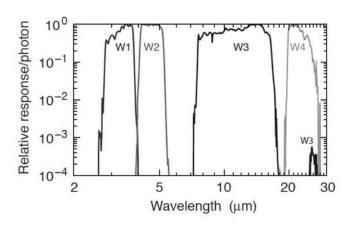
Normalized relative system response curves on a log scale. The absolute calibration is based on the Spitzer calibration (Cohen 2007).
