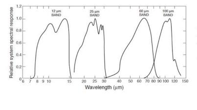
Imaging was accomplished in 4 bands: 12, 25, 60, 100  $\mu m$  as shown to the left. The filters are very broad, and so the effective wavelength of the filters depends on the spectral energy distribution of the source. Color corrections have to applied depending on whether you have a hot or cold source.
