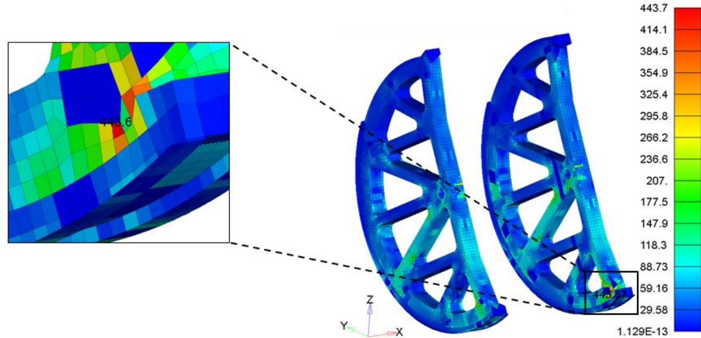
Von Mises stresses in the c-rings for elevation 30 degrees.
