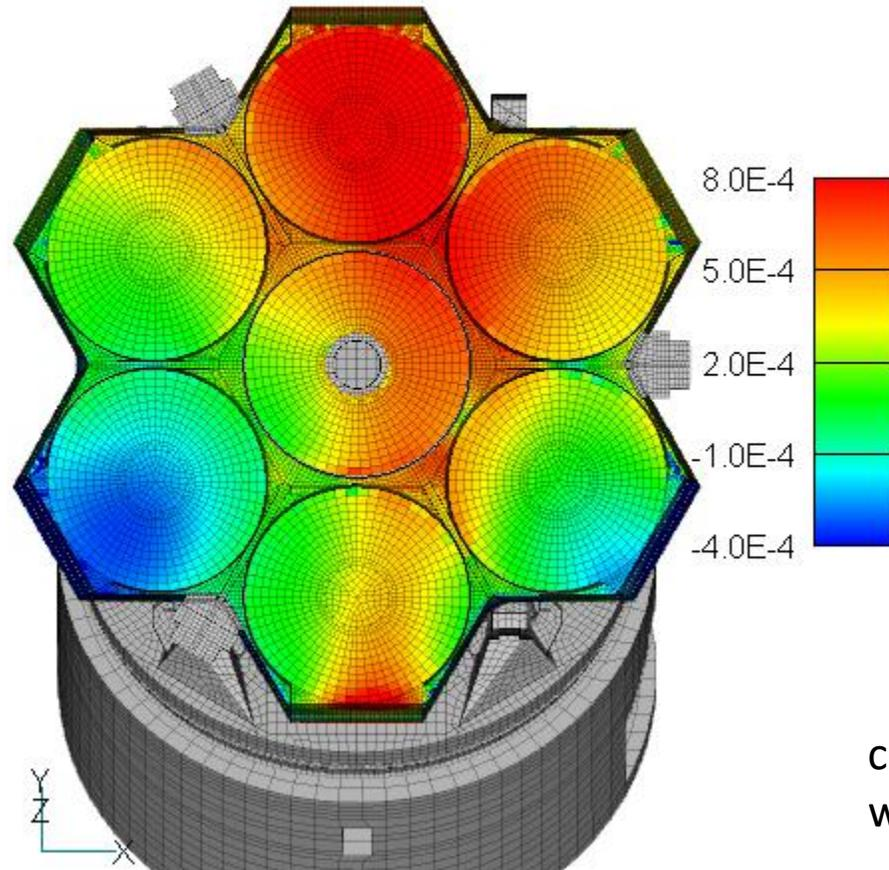
Asymmetrical secondary truss causes asymmetrical wind loading on M1.
