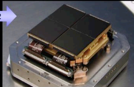
HgCdTe 4K x 4K mosaic, 18 \mu\text{m} pixels
